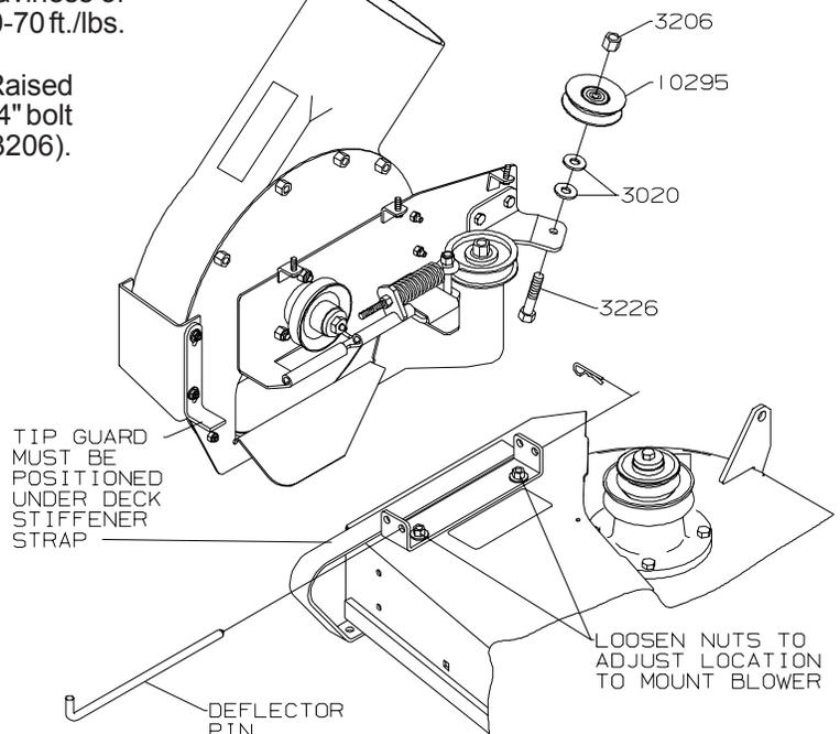
9) Slide tip guard (9884) up to contact bottom of deck stiffener and tighten nuts attaching it to the blower housing.
